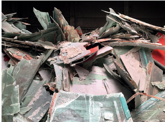
Fig. 5. Dismounted rotor blades replace traditional resources: roughly crushed and shredded, they serve as fuel and substitute for raw sand in cement factories
